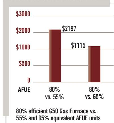
This chart depicts potential energy savings you can expect from the G50 gas furnace versus older furnaces with lower efficiency ratings. Criteria used in this example are 2,000 full-load heating hours, with a 60,000 Btuh heating design load and \$1.074 ccf for gas. Your actual savings may vary depending on the weather, local fuel rates and your lifestyle. AFUE = Annual Fuel Utilization Efficiency. Source: U.S. Environmental Protection Agency (EPA) national average energy rates.
